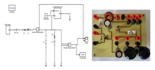
Figure 5. DC system model with RC parallel passive damping Figure 6. Hardware circuit implementation
