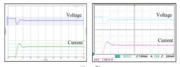
(b) (a) Figure 10. Plot of bus voltage and current with CPL= 90 W with CPL connection with passive damper; (a) simulation (b) experiment
