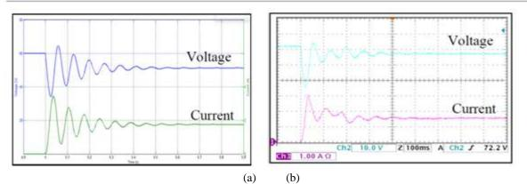
**Figure 7.** Plot of bus voltage and current with CPL= 90 W with CPL connection without passive damper; (a) simulation (b) experiment
