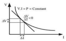
Figure 2. Negative impedance behavior of constant power load
